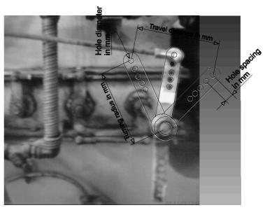
trim sledge can be fitted removing the the ball joint and refitting it on the sledge.
